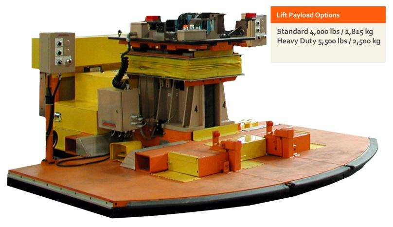
The simple construction begins with a single piece aluminum cast housing and internal components including Guide Tubes (2), Worm Gear Drive, Self-Locking Lift Chain and Servo Motor. Redundant Safeties include internal servo brake and anti-backup driving worm gear for any power interrupt and/or mechanical failure.
